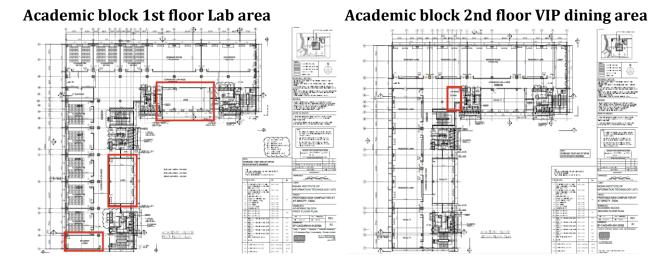
It has been decided to provide VRV system Air conditioning to the First floor (ECE Lab-1,ECE Lab-2, MEMS lab ) and Second floor (VIP Lounge/Dining area ) to use it effectively and to have easy maintenance.
